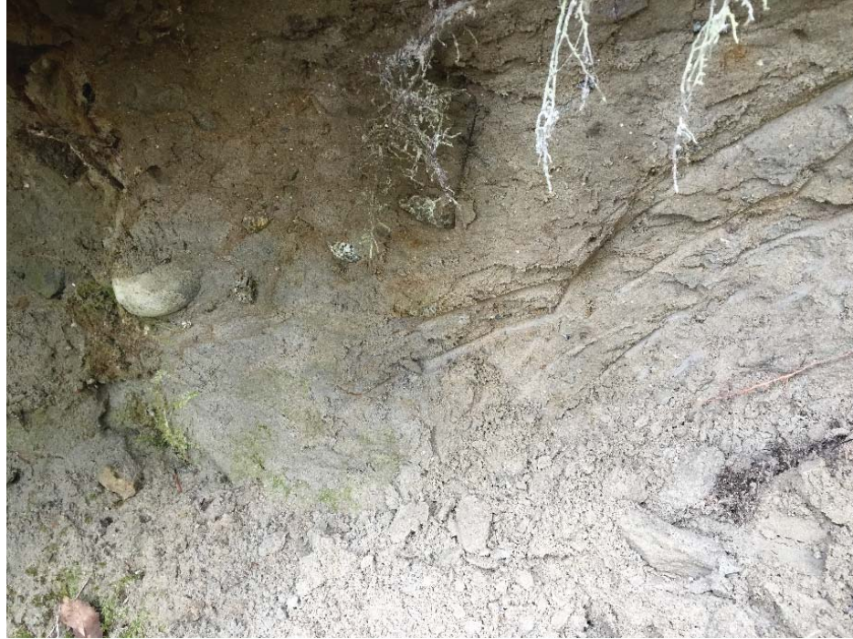
Figure 3 – Glaciofluvial deposits comprising gravelly sand with some rounded cobbles
