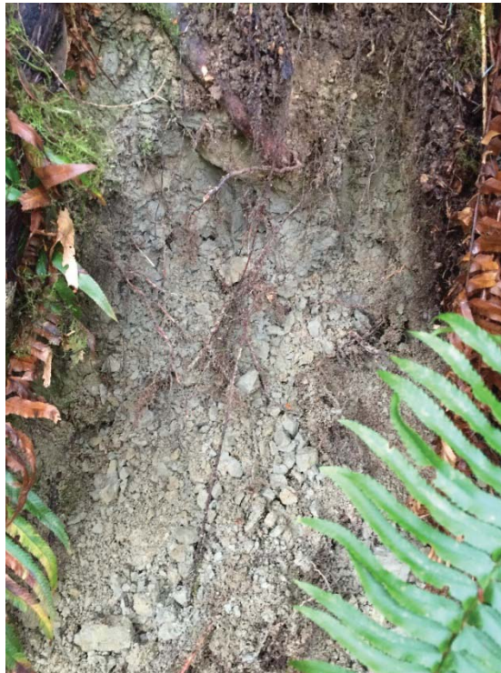
Figure 4 – Glacial till material observed along the forestry access road to the dam
