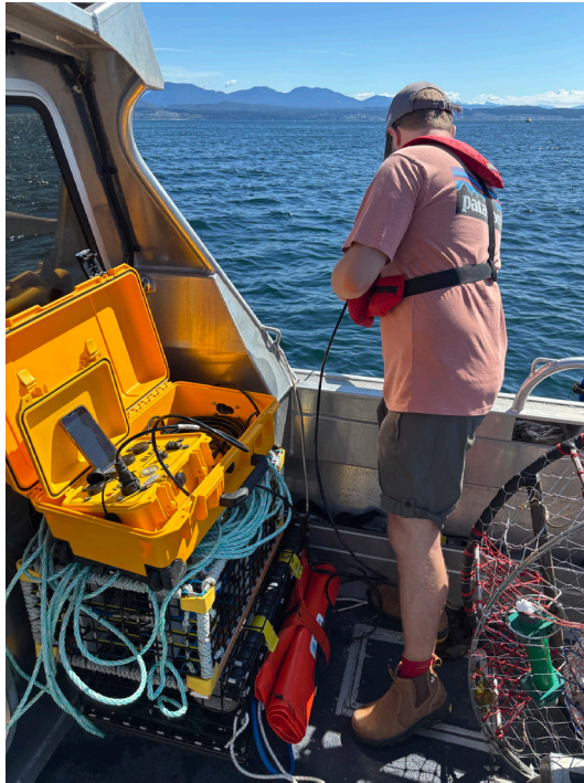
Chris Cail, a CWF summer research assistant, uses a Edgetech transducer and deckbox to send a signal to the on-demand unit in the water, in order to release the buoy that is trapped at the bottom with the on-demand unit
